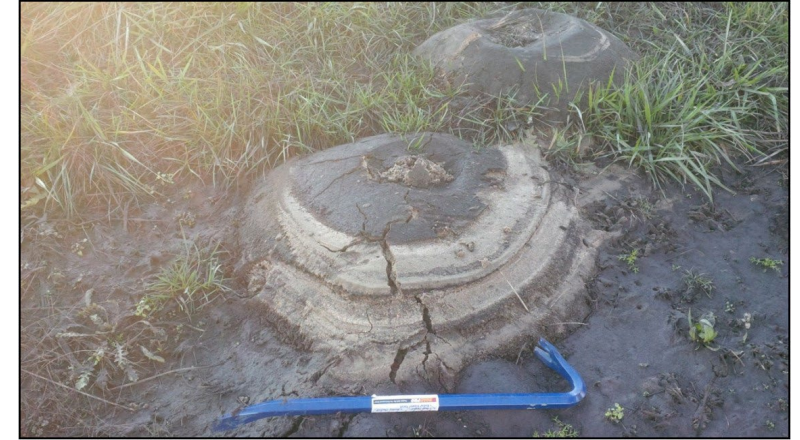
Figure 3.3. Example of sand boil, East St. Louis, 2016 New Year's Day Flood.
